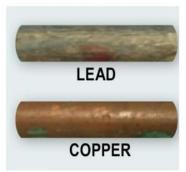
Lead: Nonmagnetic, silver-gray color. Easily scratches with a coin.
